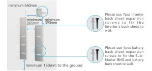
Warning: Before drilling, make sure to avoid the buried water tube and electric wires in the wall to avoid danger.
